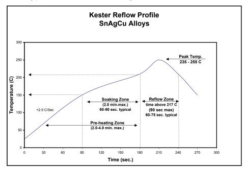
Figure 1: Recommended reflow profile using a standard reflow soldering oven
